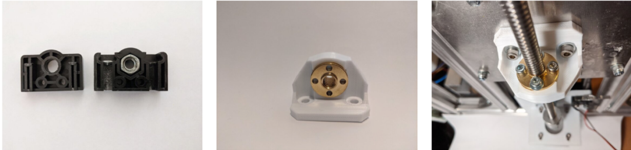
Figure 50 - Replacing the original M8 nut with an anti-backlash nut.
