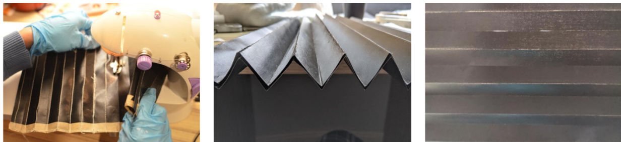
Figure 53 – Left: Sewing the bellows together with a layer of ceramic fibre in between. Middle: Folding and doubling the PTFE layers. Right: original bellows with some gaps in between.
