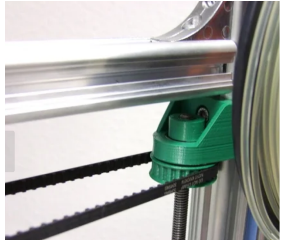
Figure 18 - Using a timing belt to synchronize z-axis movements for the other end of the K8200 printer. (55).
