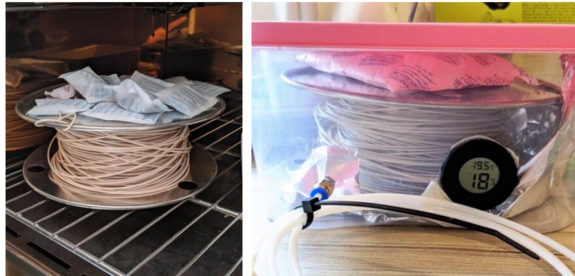
Figure 54 - Left: PEEK filament in the oven with silica gel packs. Right: PEEK in an air-tight box with packs of silica gel and a hygrometer.
