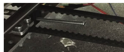
Figure 39 – Top: z-axis levelling screw when coming in contact with the z-axis endstop. Bottom: x-axis microswitch trigger.
