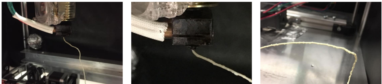
Figure 45 - First time extruding PEEK filament. The surface of the extruded line showed severe signs of blobbing and the extruded filament is abnormally wavy.
