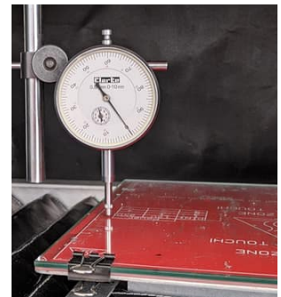
Figure 37 - DTI indicator checking for unlevel surfaces
