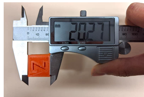
Figure 57 - Measuring the second calibration cube using a digital calliper.
